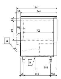
Drain Electrical inlet (power)
